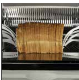
JAC FLAPS Holds the loaf together for easier handling at the exit of the machine.
